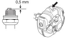
**CAUTION!** Always use the recommended spark plug type! Use of the wrong spark plug can damage the piston/cylinder.
