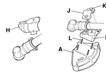
Remove the mounting plate (H). Fit the adapter (I) and bracket (J) with the two screws (K) as shown. Fit the blade guard (A) to the adapter using the 4 screws (L) as shown.
